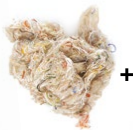
Recycled acrylic fiber from fraying is mixed with virgin solution dyed acrylic fiber
